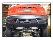
5. Install the supplied Tips (Item F) and leave them slightly loose for adjustment. Adjust the rest of the system for optimal fitment and clearance and tighten all clamps and bolts moving from front to back of the exhaust system.
