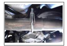
2. Using a jack-stand or muffler stand to support the factory mid-pipe, slide the supplied 3" Clamp (Item D) onto the entrance of the Y-Pipe (Item A) and then slip the Y-Pipe onto the factory mid-pipe. Be sure to locate the notch around the pin in the factory mid-pipe. Keep clamp slightly loose.
