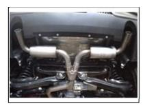
4. Install the Passenger Side Muffler Assembly (Item C) the same way you installed the Driver Side Muffler in the previous step.
